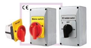
This DC isolator switch is used between DC PV arrays and grid-connected inverters. Positioned adjacent to the inverter a DC switch is required to provide a means of manually isolating the entire PV array during system installation or any subsequent maintenance.
