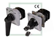
Breaker Control switches are used for tripping or closing of breakers either locally or from remote location. These switches offer advantage of having unlimited combinations of switching angles and indexing angles with stay put and spring return momentary contacts. Lost motion contacts can be cascaded, used for additional protection or for activating annunciator. The switches are modular in design hence multiple poles can be achieved as per demand of application
