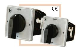
Phase Changeover Rotary Switches are used in Distribution boards. It consists of three changes over switches, each per phase, having all three phases as input. The user has a choice of changing over single phase loads using these switches. It helps to fight the common problem of phase cut in a three phase connection having single phase loads. These switches are specifically designed to fit in the distribution box having less depth to suit slimmer walls.
